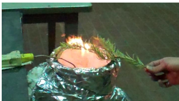
Figure 7. A grand fir branch subjected to high temperature air (650 C), explosively releasing cell contents that ignite. High-speed imagery is used to investigate convective heating.
