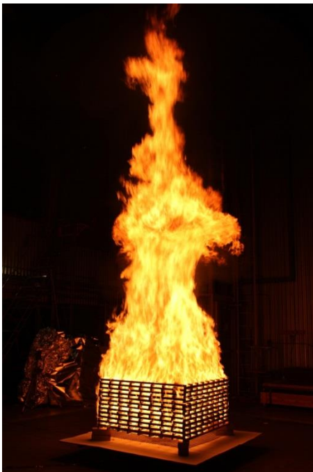
Figure 6. Photograph of large wooden crib (4'x4') burning for the study of flame structure and burning rate
