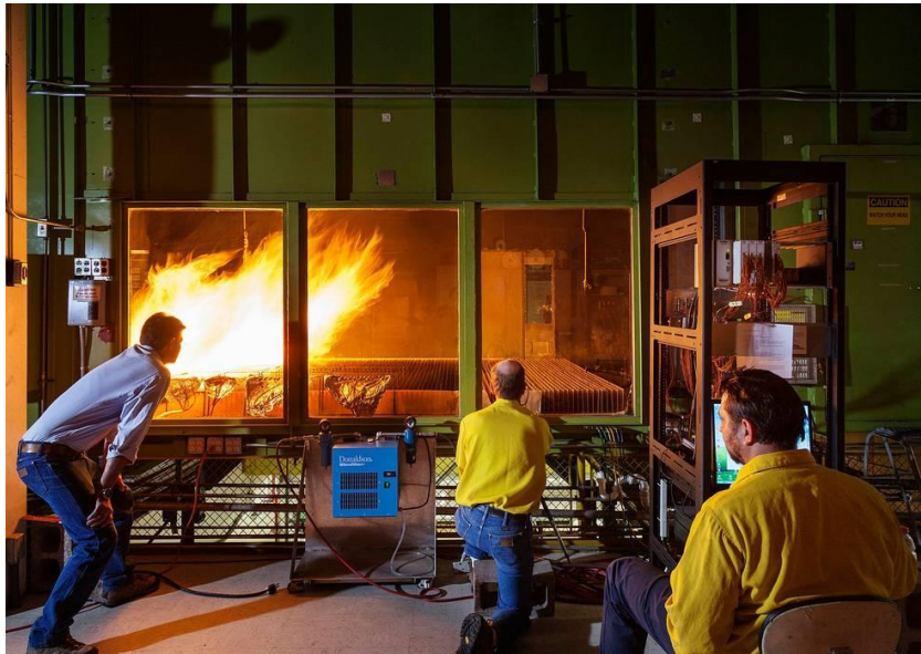
Figure 5. Photo by Richard Barnes, NY Times, showing an experimental fire burning a laser-cut cardboard fuelbed in the Missoula Fire Laboratory wind tunnel.
