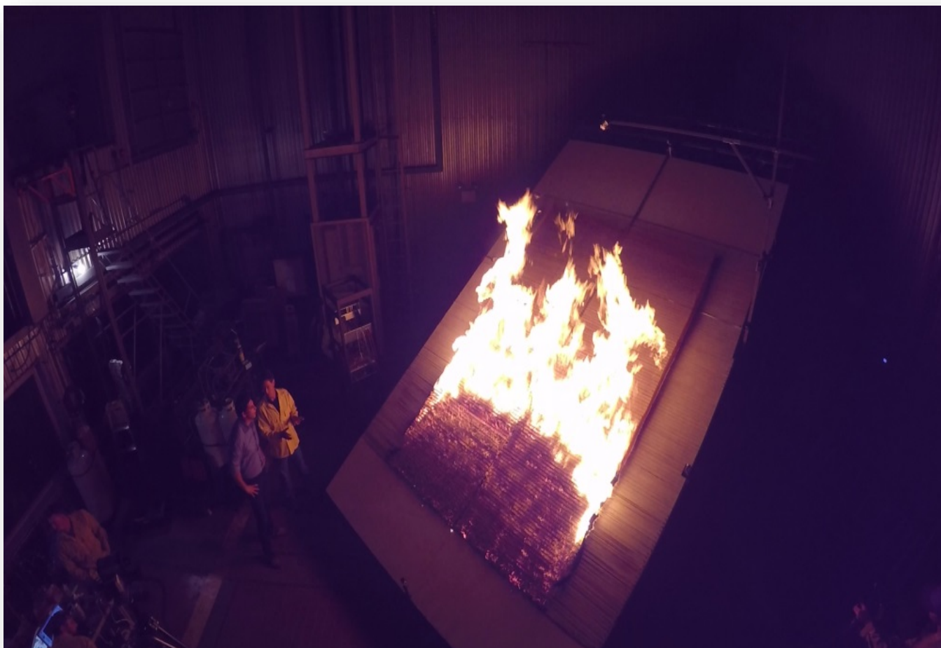
Burn experiments conducted on a tilting platform to examine slope effects on fire spread and transfer.
